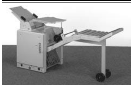
FIGURE 2 BMP with Motorised Infeed and Outfeed Conveyor
