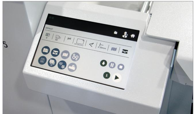
Up to 8500 A4 sheets per hour can be produced with the crease position accurate to +/- 0.004" with a maximum sheet size of 15.16" x 27.5". Up to 16 creases per sheet can be placed as close as 0.04" apart.
